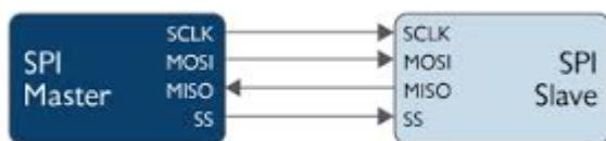
SPI connections, single slave device
