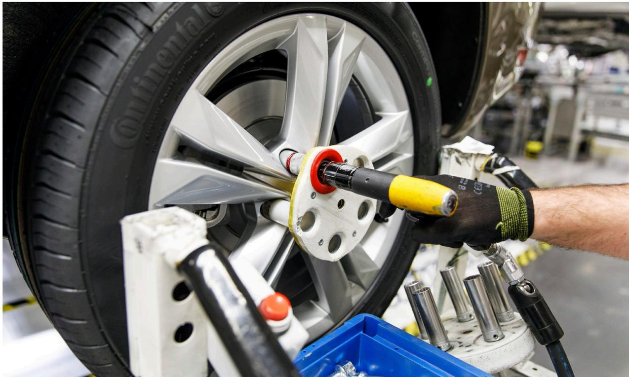
*This 3D printed wheel protection jig was previously sourced for €800, but can be 3D printed for just €21*
