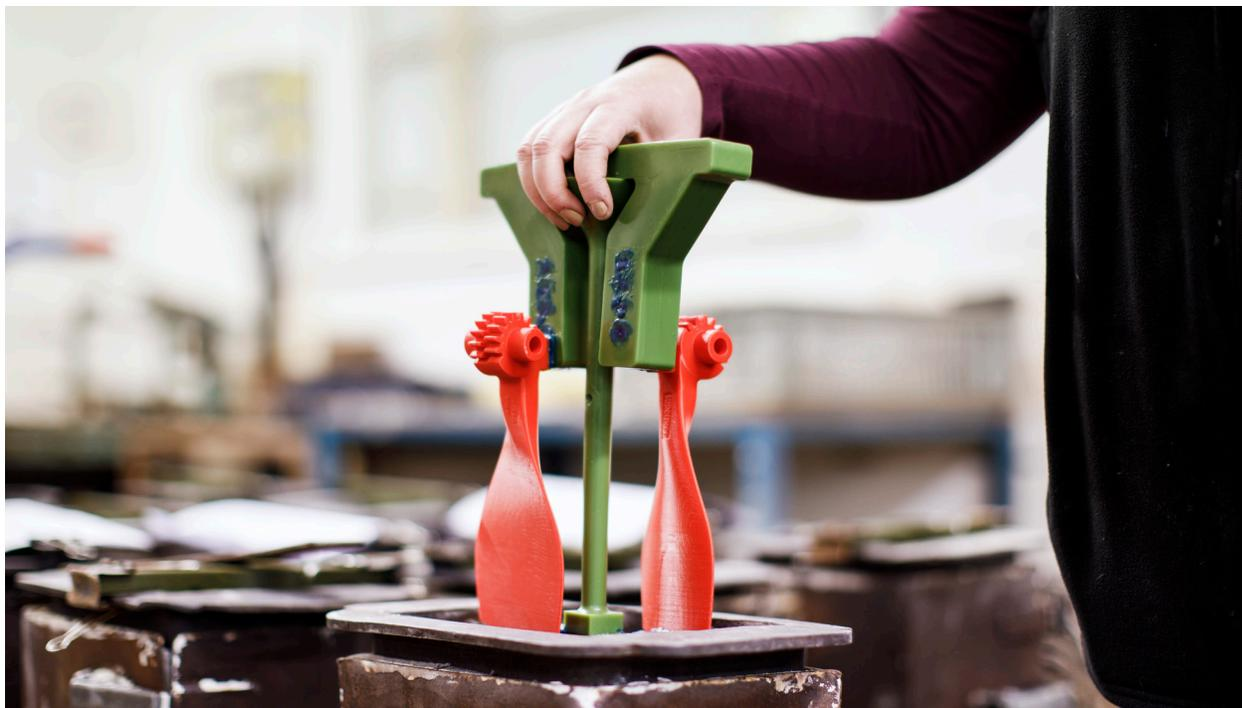
*Casting in metal from a 3D printed prototype*
