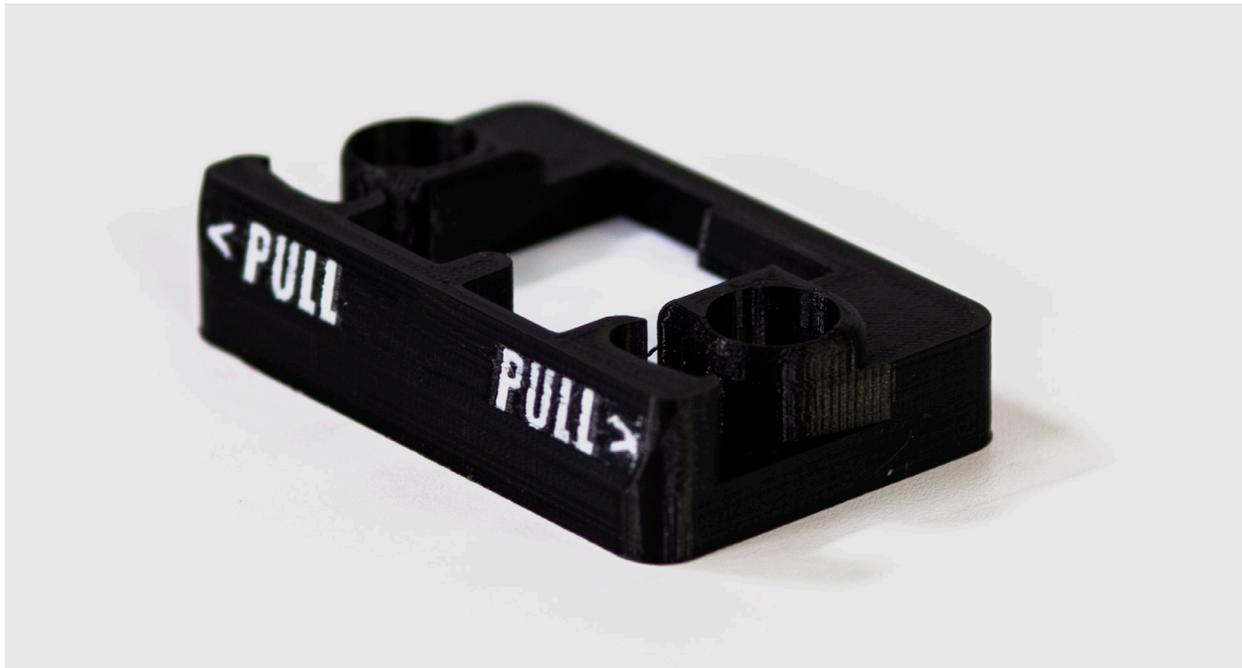
*Printing in two colors allows for clear labels to be printed directly onto parts*
